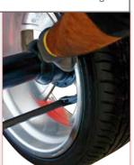
The adhesive weights can be positioned easily and rapidly using the laser line at 6 o'clock. The integrated LED light illuminates the work area to facilitate rim cleaning and application of the counterweights
