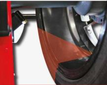
AWD automatic sensor (Auto width Device) for contactless measurement of wheel width
