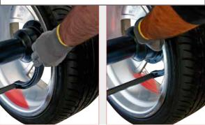
The adhesive weights can be positioned easily and rapidly using the laser line at 6 o'clock.
