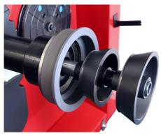
Optional : Two cone & spacer centring accessory for van light truck and off-road wheels with central hole  $\emptyset$  117÷173 mm
