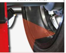
AWD automatic sensor (Auto width Device) for contactless measurement of wheel width (Xline Full Kit only)
