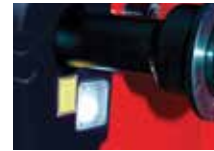
LED LIGHT ILLUMINATES THE WORK AREA
