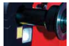
LED LIGHT ILLUMINATES THE WORK AREA
